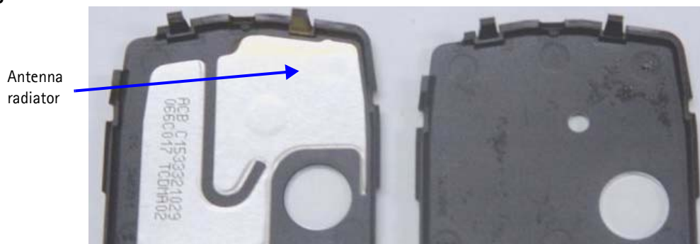
Figure 3: RM-11 phone with a missing antenna radiator
